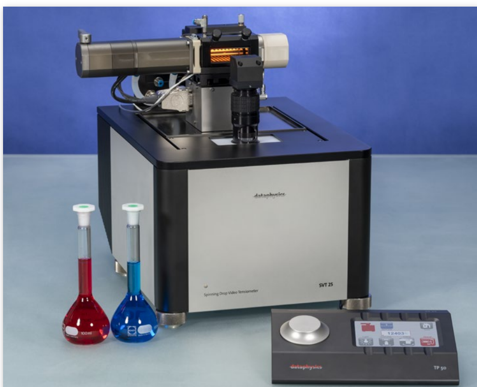
SVT 25 with temperature controlled measuring cell MC-TPC 25 and TP 50 control panel
