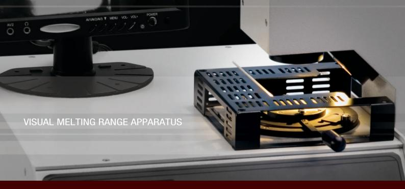
Visual Melting Range Apparatus is the latest, state-of-the-art microcontroller based instrument for determining Melting Range of white as well as coloured samples in powdered form. Around 5mg of sample is uniformly spread on a glass slide and covered with a coverslip. The slide is then placed on a specially designed uniformly heated round furnace and subjected to the heating rate specified by the user.
